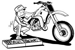
3. During disassembly, check and measure the required parts, and make a record of them so that you may refer to the record when installing them. Moreover, arrange gears, cylinders, pistons, and other parts for each section so as not to confuse or lose them.
