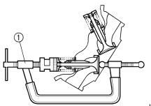
To secure the valve cotters onto the valve stem, lightly tap the valve tip with a piece of wood.
