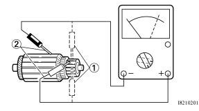
b. If any resistance is out of specification, replace the starter motor.
