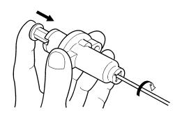
b. With the rod fully wound and the chain tensioner UP mark "a" facing upward, install the gasket "1", the timing chain tensioner "2", and the gasket "3", and tighten the bolt "4" to the specified torque.
