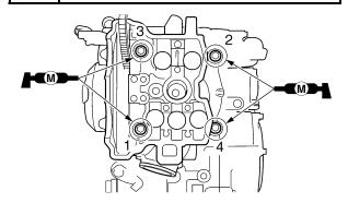
h. Put a mark on the corner "1" of the bolt (cylinder head) and the cylinder head "2" as shown.
