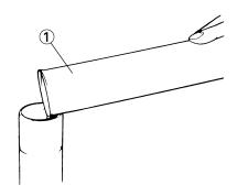
16.After filling, pump the damper rod "1" slowly up and down more than 10 times to distribute the fork oil.
