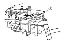
c. Remove the dowel pins and O-ring.
