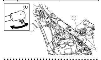
10.Put the aligning marks "a" on the throttle position sensor and carburetor.
