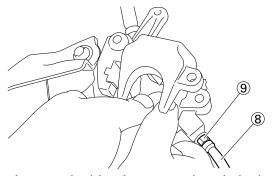
f. Loosen the bleed screw and push the brake caliper piston in.
