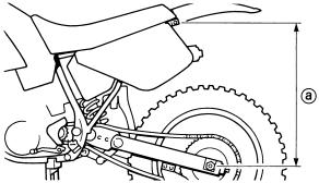
Remove the stand or block from the engine and with a rider astride the seat, measure the sunken length "b" between the rear wheel axle center and the rear fender holding bolt.
