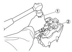
c. After installing the valve guide, bore the valve guide using a valve guide reamer "3" to obtain proper stem-to-guide clearance.
