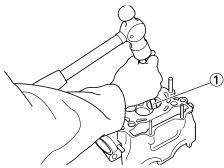
b. Install the new valve guide using a valve guide remover "1" and valve guide installer "2".
