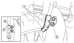
4. Pass the brake hose through the front brake hose guides "1".
