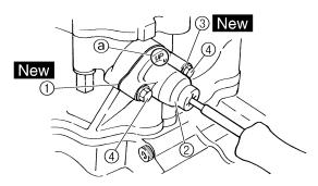
c. Release the screwdriver, check the tensioner rod to come out and tighten the gasket "5" and the cap bolt "6" to the specified torque.
