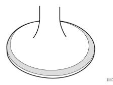
b. Apply molybdenum disulfide oil to the valve stem.
