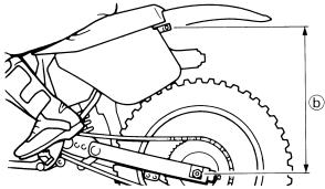
Loosen the locknut "1" and make adjustment by turning the spring adjuster "2" to achieve the standard figure from the subtraction of the length "b" from the length "a".
