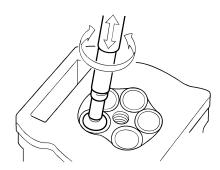
e. Apply a fine lapping compound to the valve face and repeat the above steps.
