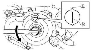
c. Fit the timing chain "3" onto both camshaft sprockets and install the camshafts on the cylinder head.
