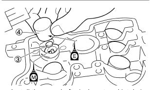
g. Install the camshafts (exhaust and intake). Refer to "CAMSHAFTS" section in the CHAPTER 5.
