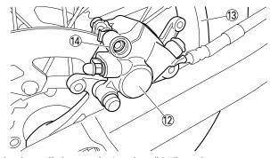
k. Install the pad pin plug "15" and protector "16".
