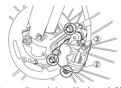
d. Remove the pad pin and brake pads "4".
