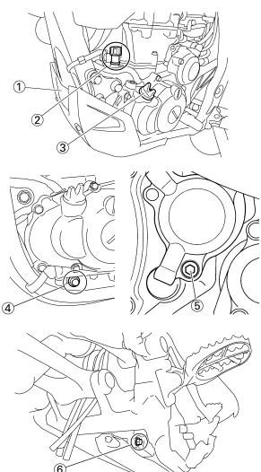
4. If the oil filter is to be replaced during this oil change, remove the following parts and reinstall them.
