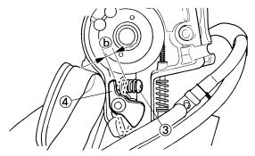
c. Gradually turn out the adjusting screw while moving the link lever until it has no more free play.
