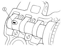
c. Install the clip, dowel pins and camshaft caps.
