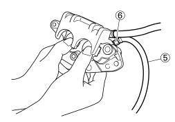
f. Loosen the bleed screw and push the brake caliper piston in.
