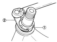
Check the steering stem by turning it lock to lock. If there is any binding, remove the steering stem assembly and inspect the steering bearings.
