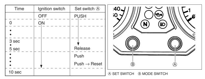
Pointer will return to the starting point right after the completion of the operation. In the case of the pointer not returning to the proper position after doing above, replace the combination meter unit.
