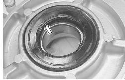
• Remove the dust seal with the special tool.
