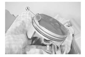
• Apply a light coat of molybdenum oil solution to the piston pin.
