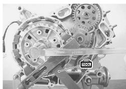
• Lock the clutch sleeve hub nut with a center punch.
