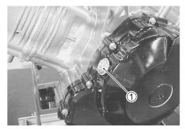
• Apply engine oil to the new O-ring and install the generator cover plug.
