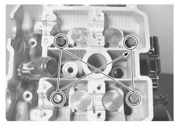
• After firmly tightening the cylinder head bolts (M10), install the cylinder head nuts and bolts.
