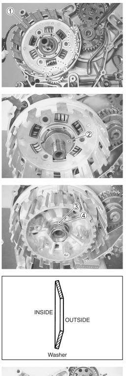
• Tighten the clutch sleeve hub nut to the specified torque with the special tool.
