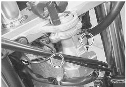
Inspect each switch for continuity with a tester. If any abnormality is found, replace the respective switch assemblies with new ones.
