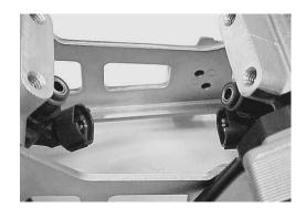
• Connect the fuel injector couplers to the fuel injectors.
