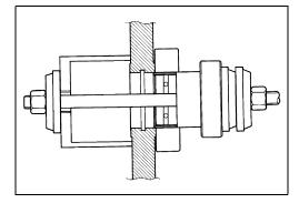
• After installing the bearings, check the bearing surface for any scratch or damage.
