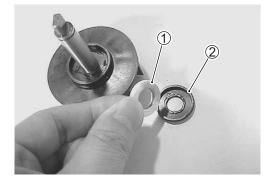
Remove the snap ring from the impeller shaft.Remove the impeller from the other side.
