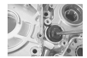
• Remove the oil seal with the special tool.
