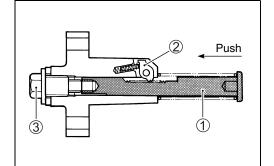
• From this position, turn out the cam chain tension adjuster bolt ③ until locking the cam chain tension adjuster rod ①. Now the cam chain tension adjuster is ready to install.
