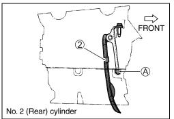
• Tighten the cam chain tensioner mounting bolts to the specified torque.
