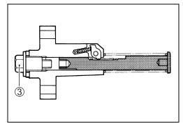
• Compress the cam chain tension adjuster rod ① fully by releasing the ratchet ②.
