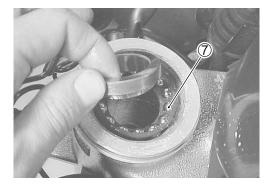
• Remove the steering stem lower bearing (8).
