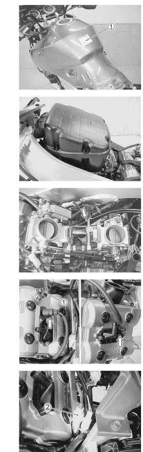
• Disconnect the generator lead wire coupler ① and signal generator lead wire coupler ② by removing the screw ④.
