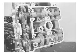
• Install the dowel pins.
