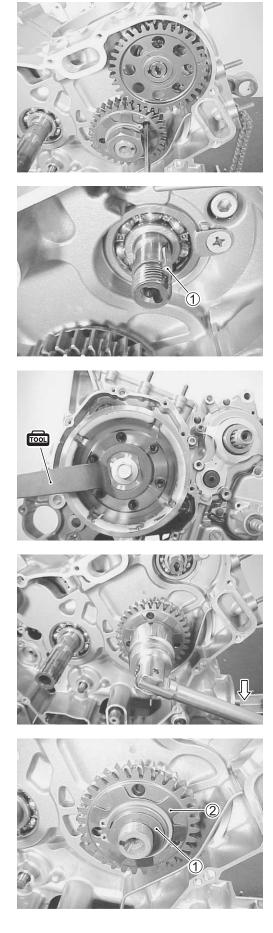
• Remove the key 1 and thrust washer 2.
