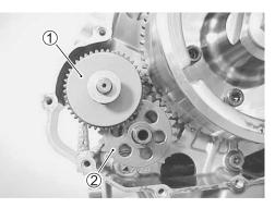
• Remove the bushings ① from the crankcase and generator cover.
