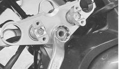
• Remove the handle holder nuts ④ and disassemble the handle holder.
