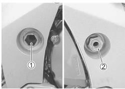
• Tighten the swingarm pivot lock nut to the specified torque with the special tool.
