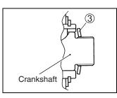
• Install the primary drive gear nut.
