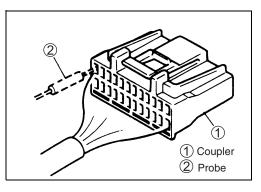
• When taking measurements at electrical connectors using a tester probe, be sure to insert the probe from the wire harness side (backside) of the connector/coupler.
