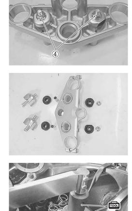
• Remove the steering stem nuts with the special tools.
