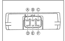
Measure the voltage between the terminals using the multi circuit tester as indicated in the table below. If the voltage is not within the specified value, replace the regulator/rectifier with a new one.
