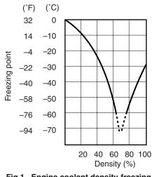
Fig.1 Engine coolant density-freezing point curve.
