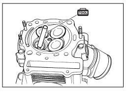
If the contact area is too high on the valve, or if it is too wide, use the  $15^{\circ}/60^{\circ}$  cutters (for exhaust side) and  $30^{\circ}/60^{\circ}$  cutters (for intake side) to lower and narrow the contact area.
