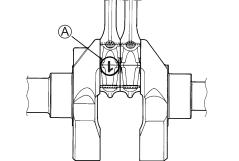
Apply engine oil to the bearing cap bolts.
