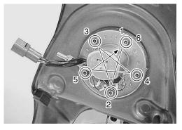
① Fuel pressure regulator 2 Fuel pump case/Fuel filter cartridge (5) (For high pressure) ③ Fuel pump ④ Fuel mesh filter (1)(For low pressure) 5 Fuel level gauge ₽' 2 503 . J<sub>w</sub> 3 (4) 10 N·m (1.0 kgf-m, 7.3 lb-ft) 10 Æ∂ H
