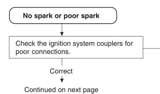
\* Check that the transmission is in neutral and the engine stop switch is in the "RUN" position. Pull the clutch lever. Check that the fuse is not blown and the battery is fully-charged before diagnosing.
