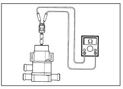
Check the resistance between the terminals of the PAIR control solenoid valve.
