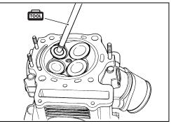
• The ring-like dye impression left on the valve face must be continuous without any break. In addition, the width of the dye ring, which is the visualized seat "width", must be within the following specification:
