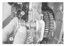
• Check and correct the positions of the "F I T" line on the generator rotor and cam drive idle gear/sprocket ①.
