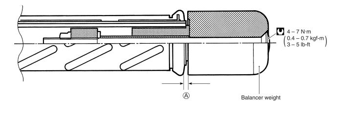
LH clearance A is 0 mm. RH clearance A is 0.5 – 1.5 mm.
