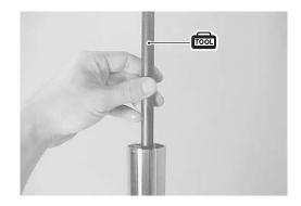
• Install the fork spring. NOTE: The smaller end of the fork spring should be at the bottom of the front fork.
