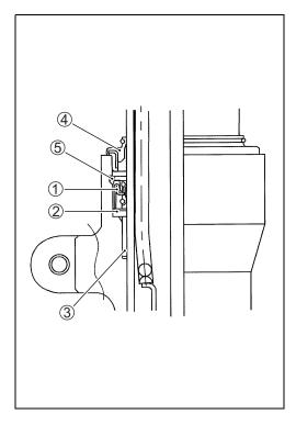
• Insert the inner tube into the outer tube and fit the oil seal and dust seal with the special tool.
