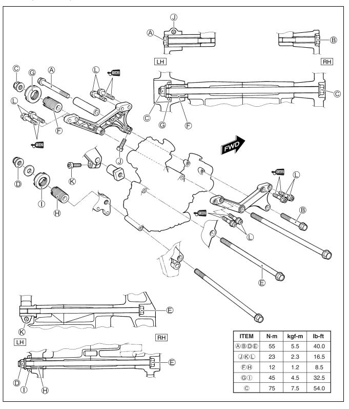
• Before installing the engine assembly, install the spacer (A), collar (B) and engine thrust adjuster (C), (D).
