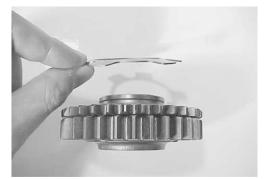
• Install the snap ring ① completely with the special tool.
