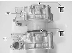
• Hold the piston rings in proper position, and insert each of the pistons into the respective cylinders.
