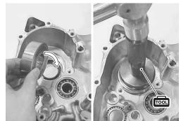
• Install the bearing retainers.
