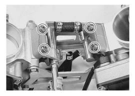
• Remove the fuel injectors.
