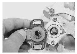
• With the TV fully closed, install the TP sensor.
