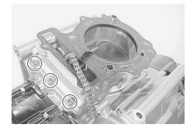
• Remove the cylinder base gasket and dowel pins.
