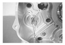
• Install the gear position switch and cable guide.
