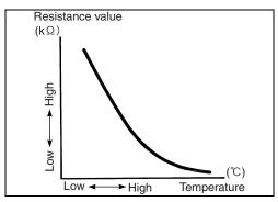
**ENGINE COOLANT TEMPERATURE SENSOR (ECT SENSOR)** The engine coolant temperature sensor is installed at the thermostat case.
