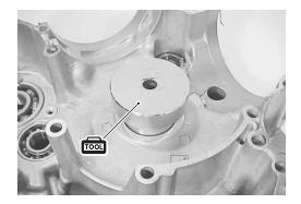
• Gradually press out the bearing with the special tool by using the hand-press.
