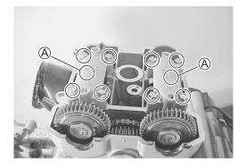
• After installing the No.2 (Rear) camshafts, rotate the generator rotor 360 degrees (1 turn), and recheck the positions of the camshafts.
