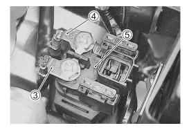
Apply 12 V to A and B terminals and check for continuity between the positive and negative terminals using the multi circuit tester. If the starter relay clicks and continuity is found, the relay is ok.
