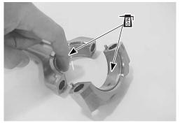
• When fitting the conrods on the crankshaft, make sure that I.D. codes (A) of the conrods face each cylinder intake valve sides.
