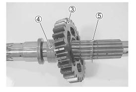
• When installing a new snap ring, pay attention to the direction of the snap ring. Fit it to the side where the thrust is as shown in the figure.
