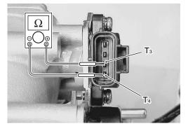
If the measured resistance is not within specification, adjust the STV adjuster (A) as follows:
