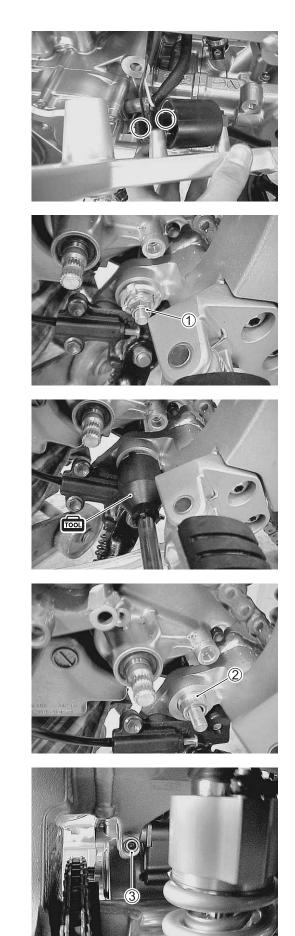
Gradually lower the engine assembly by removing the bolt ①,
