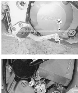
• Adjust the gearshift lever as shown.
