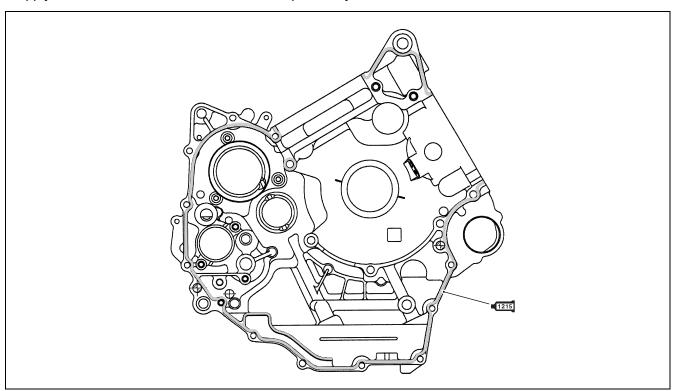
When securing the right and left crankcase halves, tighten each bolt a little at a time to equalize the pressure. Tighten all the securing bolts to the specified torque values.
