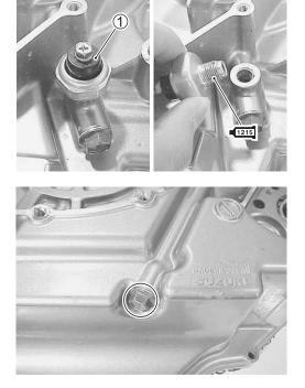
• Remove the oil jet with a suitable bar.
