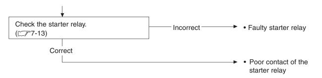
The starter motor runs when the transmission is in neutral with the side-stand up or down, but does not run when the transmission is in any position other than neutral with the side-stand down.
