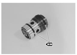
• Reinstall the compression adjuster assembly ①.
