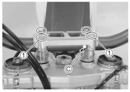
Tighten the handlebar holder set nuts to the specified torque.
