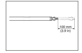
• Make sure approx. 10 mm (0.39 in) of inner rod thread is exposed on the end.
