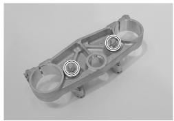
• Remove the handlebar holders, damper bushings and spacers.
