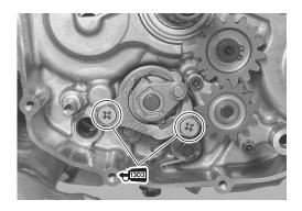
Install the gearshift return spring <sup>(1)</sup>/<sub>(4)</sub>, snap ring <sup>(5)</sup>/<sub>(5)</sub> and washer <sup>(6)</sup>/<sub>(6)</sub> onto the gearshift shaft <sup>(3)</sup>/<sub>(3)</sub> properly.
