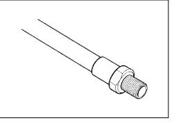
• With the damper rod held in vertical position, compress the damper rod fully to discharge an excess of oil.
