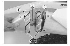
• The rear muffler body mounting bolt is of flanged type which tightens the muffler body ④, rear muffler body ① and inner plate ② together. When tightening, make sure to properly align the screw holes of these three parts to prevent the bolt from cross-threading or interfering with the screw holes.
