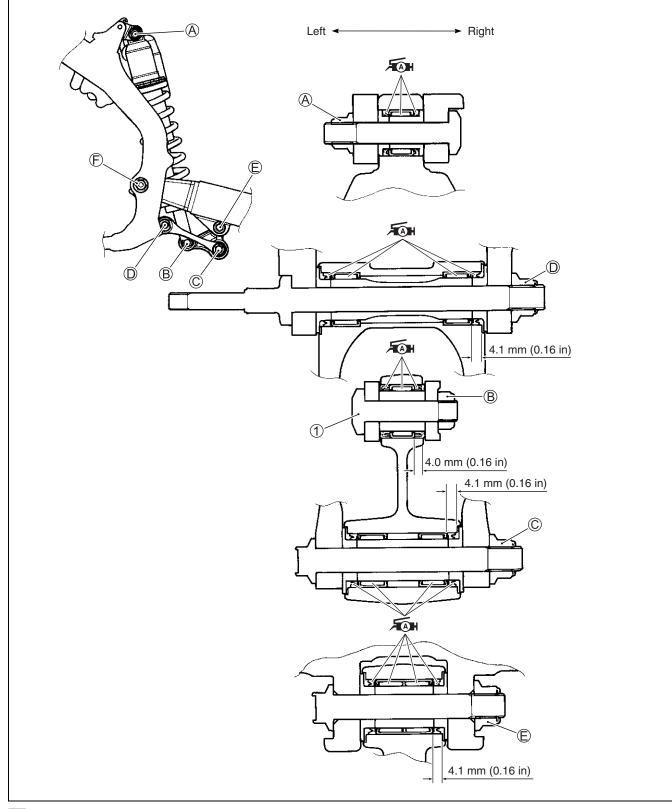
• Tighten the cushion lever, cushion rod and swingarm nuts to the specified torque.
