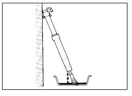
• Force out the remaining oil using compressed air completely.
