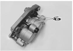
• Tighten the caliper mounting bolts ① to the specified torque.
