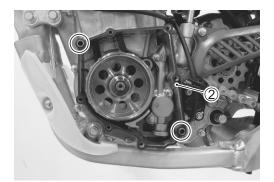
• Install the magneto cover ③ and magneto cover guard ④.
