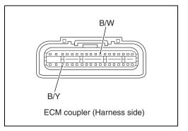
• Measure the engine stop switch resistance between B/Y lead wire and B/W lead wire.
