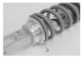
• Adjust the spring set length and tighten the lock-nut.
