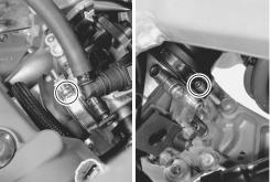
• Remove the fuel delivery pipe 6.
