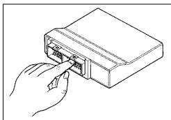
• When disconnecting and connecting the ECM, make sure to stop the engine, or electronic parts may get damaged.
