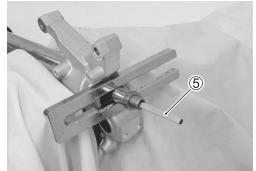
• With the outer tube compressed by hands, remove the special tool.
