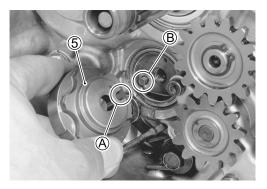
• Apply a small quantity of THREAD LOCK to the gearshift cam driven pin (6) and tighten it to the specified torque.
