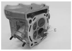
• Remove the valve stem seal  $\overline{\mathcal{T}}$  and spring seat  $\underline{\$}$ .
