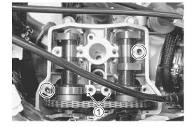
• Apply grease to the new O-ring and install it to the camshaft journal holder.
