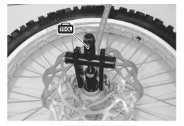
• Install new bearings with the special tool, using the suitable spacer (A) match for the outside dimension of bearings.
