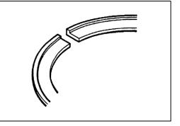
• Position the gaps of the two ring as shown. Before inserting a piston into the cylinder, check that the gaps are so located.
