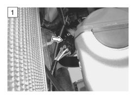
3) Disconnect the CKP sensor coupler and measure the resistance.
