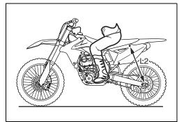
After the sag measurement has been set 100 mm (3.94 in), test ride the motorcycle and adjust the suspension for the rider and track conditions referring to the guide below.
