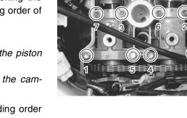
• Install the gasket (5) and cam chain tension adjuster cap bolt (6).
