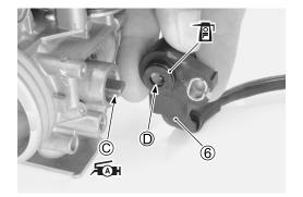
• Align the groove of hot starter valve with the hot starter cable end.
