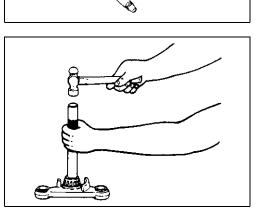
• Drive out the outer races using the steel rod.
