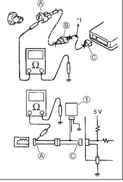
① Other parts \*1 To other parts • Disconnect the connector/coupler included in circuit (coupler (B)) and measure resistance between terminal (A) and body ground.
