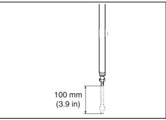
• Tighten the lock-nut by hand completely.
