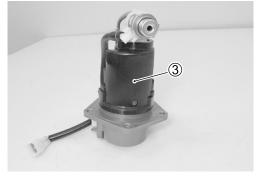
• When installing the fuel pump assembly, first tighten all the fuel pump mounting bolts lightly and then to the specified torque.
