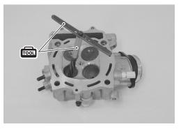
Cool down the new valve guides in a freezer for about one hour and heat the cylinder head to 100 – 150 °C (212 – 302 °F) with a hot plate.
