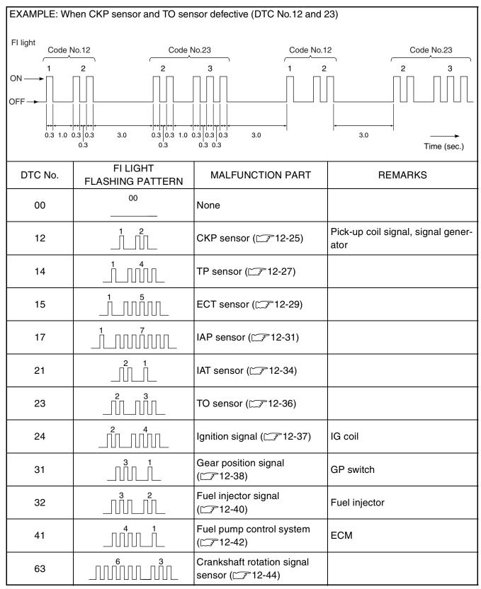
In the FI light, the DTC is indicated from small code to large code.
