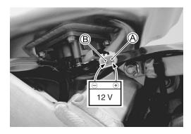
• Connect a proper lead wire into the fuel pump coupler (fuel pump side) and apply 12 volts to the fuel pump (between terminal (A) and terminal (B) for 10 seconds and measure the amount of fuel discharged.
