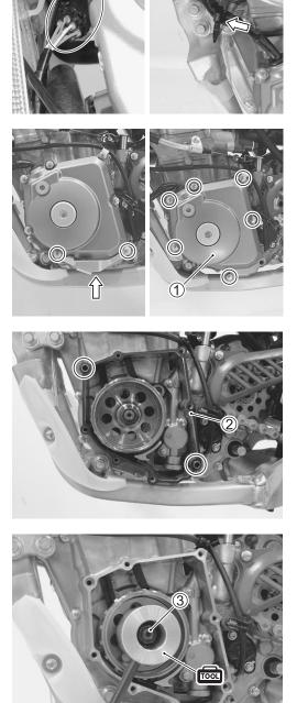
• Remove the magneto rotor ④ with the special tool.
