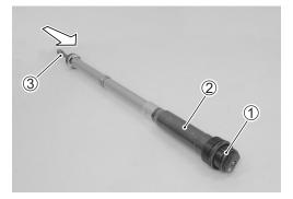
• Drain the fork oil from the damper rod assembly by moving the inner rod several strokes.
