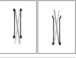
• Fit the upper and lower outer races with the special tools.
