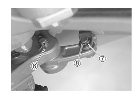
Install the kick starter lever in the correct position. ( 38-7)
