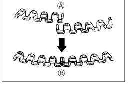
• Be sure to bring the concave side of 1st ring to the top when fitting it to the piston.
