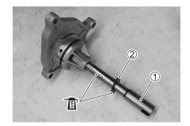
• Apply molybdenum solution to the impeller shaft ① and washer ②.
