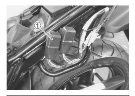
First, check for insulation with the tester between terminals (A) and B. Next, check for continuity between A and B with 12 V voltage applied, positive  $\oplus$  to terminal  $\mathbb C$  and negative  $\oplus$  to terminal D. If continuity does not exist, replace the fuel pump relay with a new one. 09900-25008: Multi circuit tester set
