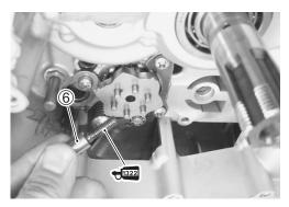
• Install the gearshift shaft assembly  $\overline{\mathcal{O}}$  with the washer  $\underline{\otimes}$ .
