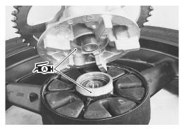
• Tighten the rear sprocket nuts to the specified torque.
