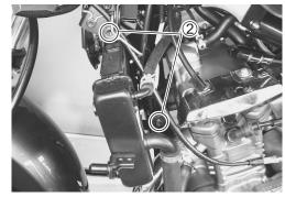
Apply thread lock to the reservoir tank mounting bolts ③ and tighten them to the specified torque as shown in the cooling system hose routing. (17710-20)
