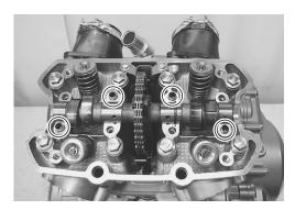
• Turn the crankshaft counterclockwise and remove the camshaft sprocket bolts (9).
