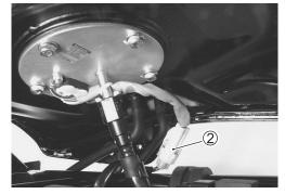
• Disconnect the fuel pump lead wire coupler 2.
