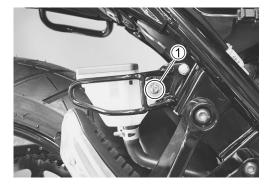
• Place a clean rag underneath the union bolt ② on the master cylinder to catch spilled drops of brake fluid.
