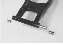
• Remove the swingarm pivot bearings ① using the special tools.
