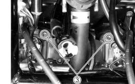
• Equalize the vacuum of the cylinders by turning each air screws (3) and keep it running at idling speed.
