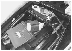
• Install the TO sensor in the reverse order of removal. (13710-39)
