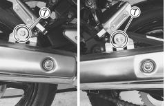
• Remove the each part from the muffler as shown in the exhaust system components. (2710-27)
