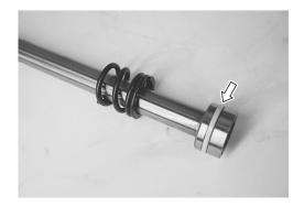
Insert the inner tube into the outer tube and install the oil seal
