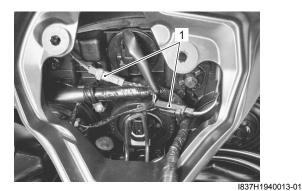
5) Remove the rear view mirror/turn signal assemblies.
