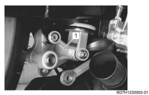
6) Remove the rear shock absorber upper mounting bolt and nut.
