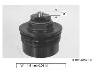
6) Slowly turn the cap bolt completely by hand until the end of the cap bolt seats on the inner-rod.
