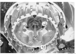
11) Unlock the clutch sleeve hub nut.
