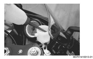
4) Fill the reservoir with new brake fluid.
