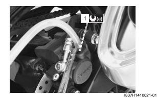
9) Fill the reservoir with brake fluid to the upper mark of the reservoir.
