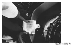
5) Fill the reservoir with new brake fluid.
