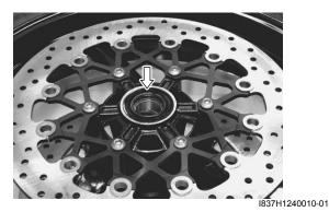
Wheel Axle Using a dial gauge, check the wheel axle for runout. If the runout exceeds the limit, replace the axle shaft.
