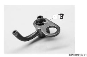
· Install each piston cooling oil jet.
