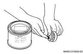
2) Install the bearing (1) and dust seal (2) to the sprocket mounting drum with the special tools.
