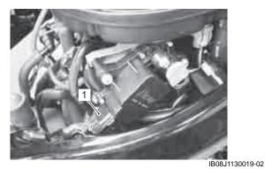
3) Connect the special tool between the STP sensor and its coupler.
