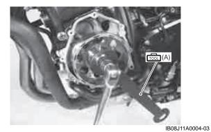
9) Install a bolt "A" of suitable size to the left end of crankshaft.
