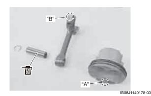
• Install the new piston pin circlips (1).
