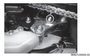
4) Remove the rear shock absorber upper mounting bolt and nut.
