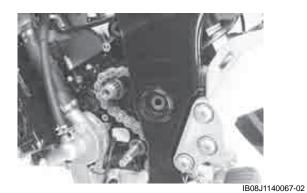
Install all engine mounting bolts and tighten them temporarily.
