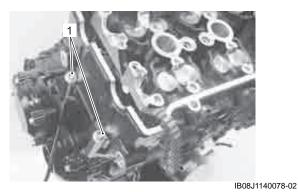
2) Remove the cylinder head bolts and washers.
