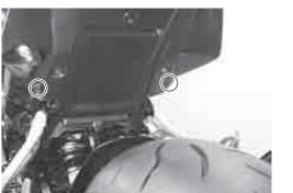
7) Remove the frame cover assembly from the frame.
