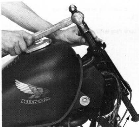
BEARING RACE REMOVER/INSTALLER 07946-3710400
