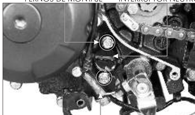
CABLE CONECTOR DEL INTERRUPTOR NEUTRO
