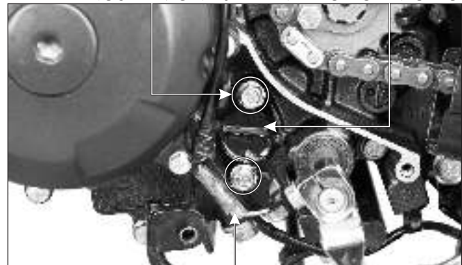
CABLE CONECTOR DEL INTERRUPTOR NEUTRO
